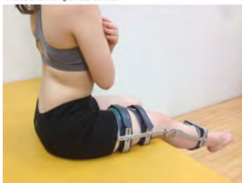
Figure 1. Standardization of knee flexion/extension angle during measurement using a metal orthosis.
