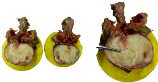
Figure 3: Left) Transverse section through a disc following 100 000 cycles of loading. Right) Both the nucleus replacement (tweezer tip) as well as the annulus repair device are still contained within the disc periphery on the posterior right hand aspect of the annulus.
