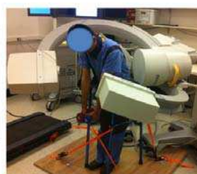
Fig 2: Dual fluoroscopic imaging system for in vivo testing of weightbearing standing position.
