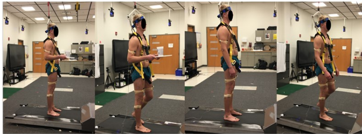
Figure 1. The experimental protocol used a treadmill to produce a perturbation while a subject with low back pain was in a quiet standing posture. Each subject was protected by a full-body safety harness during trials on the treadmill. A: a subject holding a tray, B: a subject not holding a tray during the perturbation trial.
